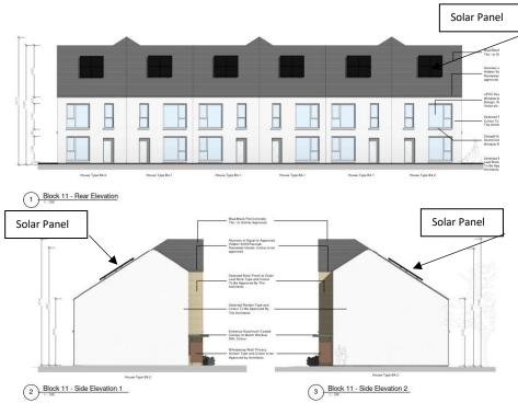
Figure 2: Extract from drawing no. 1757-PA-202 Block 11 demonstrating house design addressing link street – three storey fronting link street and two storey to the rear.
